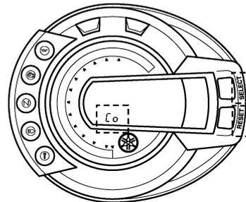
5. After selecting the cylinder, simultaneously press the "SELECT" and "RESET" buttons for 2 seconds or more to execute the selection.
