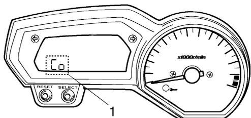
4. After selecting “Co”, simultaneously press the “SELECT” and “RESET” buttons for 2 seconds or more to execute the selection.
