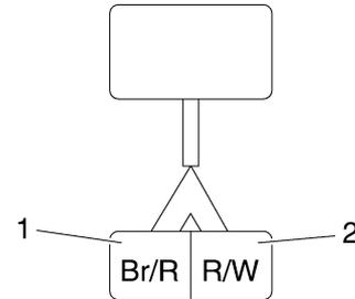
c. Measure the air induction system solenoid resistance.
