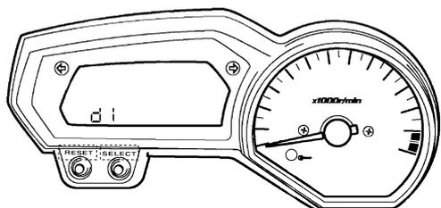
3. Press the “SELECT” button to select the CO adjustment mode “Co” “1” or the diagnostic mode “dl”.
