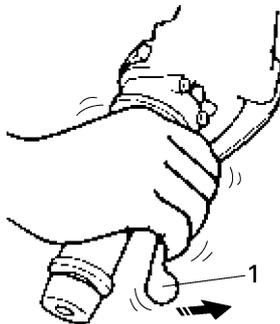
10. After the pulsating action has stopped in the brake lever, it is generated in the brake pedal "2" 0.5 second after and continues for approximately 1 second.
