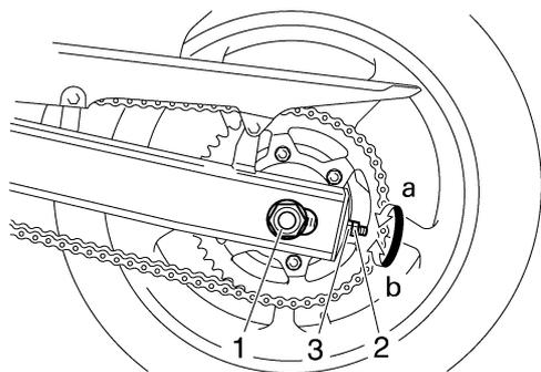
d. Tighten both locknuts to specification.
