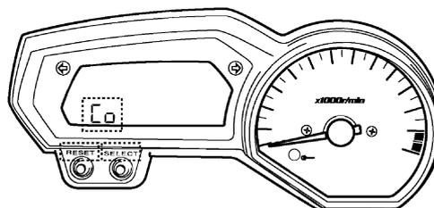
5. After selecting the cylinder, simultaneously press the “SELECT” and “RESET” buttons for 2 seconds or more to execute the selection.
