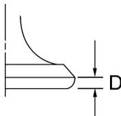
Valve stem diameter (intake)
