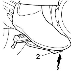
11. After the pulsating action has stopped in the brake pedal, it is generated in the brake lever 0.5 second after and continues for approximately 1 second.
