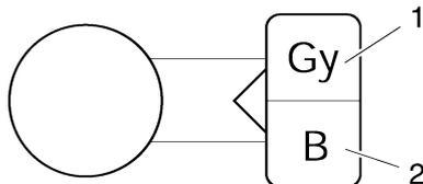
b. Measure the crankshaft position sensor resistance.
