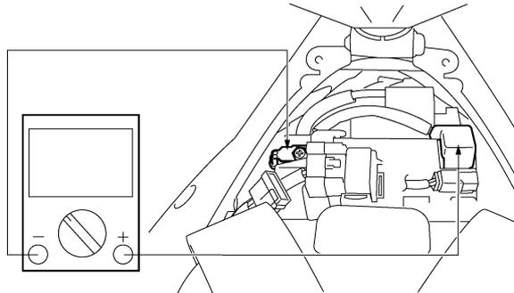
**Malfunction code 52 (Rear wheel will not recover from the locking tendency even though the signal is continuously transmitted from the ABS ECU to release the hydraulic state [when the battery voltage is low].)**
