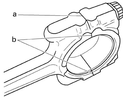
e. Tighten the connecting rod bolts.
