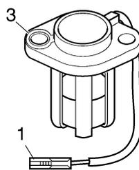
b. Measure the pickup coil resistance.
