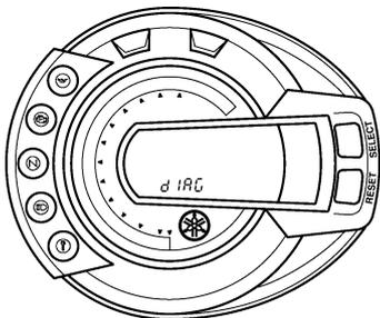
3. Press the "SELECT" button to select the CO adjustment mode "Co" "1" or the diagnostic mode "dl".
