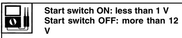
Out of specification → Replace the handlebar switch.
