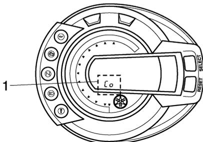
4. After selecting "Co", simultaneously press the "SELECT" and "RESET" buttons for 2 seconds or more to execute the selection.
