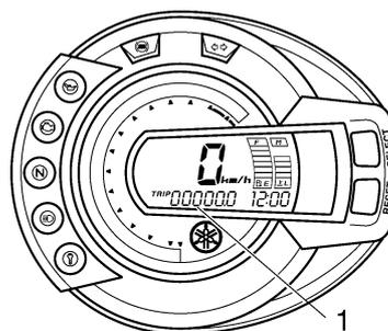
1. Odometer/tripmeter/fuel reserve tripmeter/tachometer
